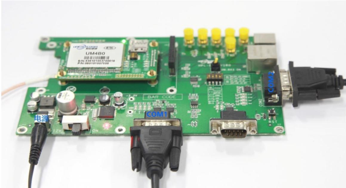
Figure 4-3 Connect the Serial Port
